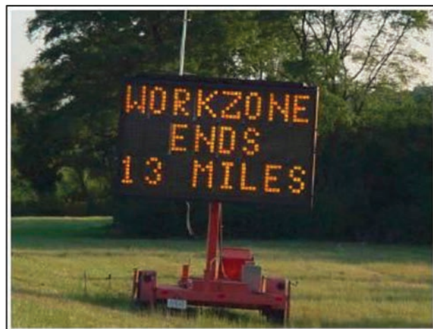
Figure 3.17 Changeable message sign in TIPS system displaying distance to the end of the work zone (Zwahlen, 2002).
