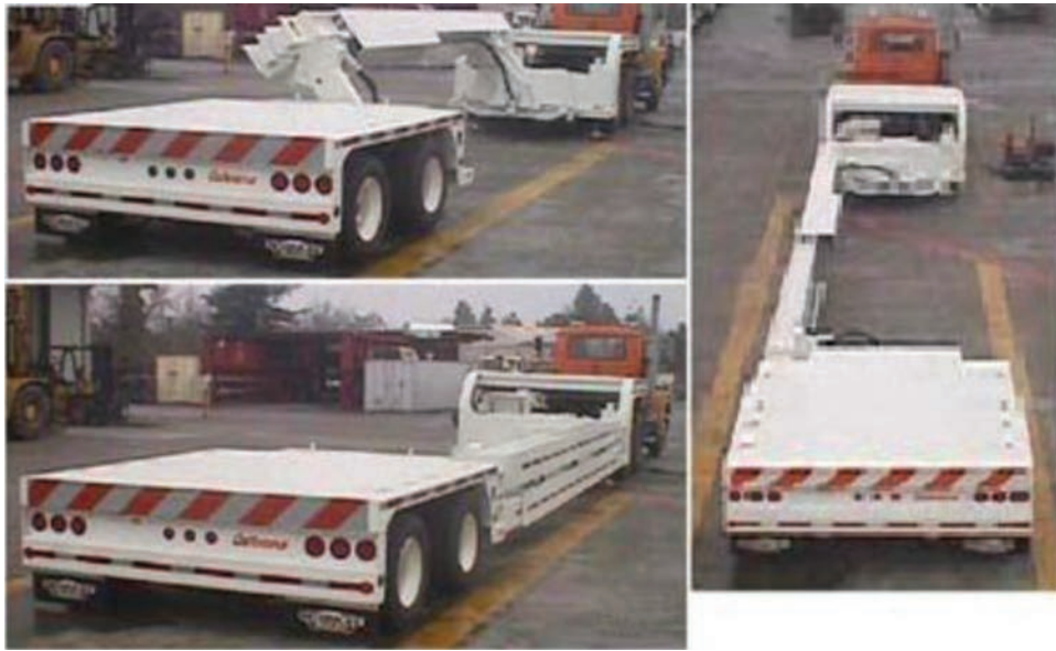
Figure 3.37 Balse Beam mobile barrier system (California Department of Transportation, 2010).
