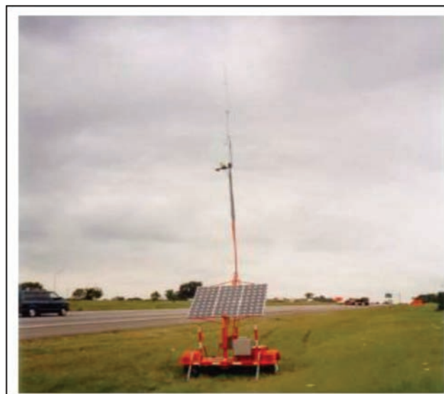
Figure 3.18 Sensor station trailer configured with traffic sensor, microwave antenna and solar panel (Zwahlen, 2002).
