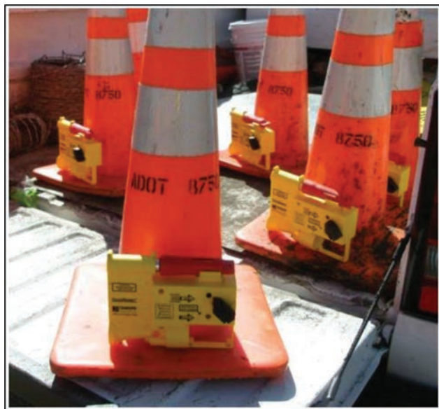
Figure 3.15 SonoBlaster!® Work Zone Intrusion Alarm (Krupa, 2010).
